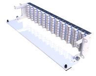
2U Ultra High Density (UHD) Patching Frame is the part of the system for high density fiber optics infrastructure management in Data Centres and Telecommunication environments. 2U frame can house up to 12 x UHD Patch Adapter Plates- design allows to scale up to 288x LC and 144x SC ports.
